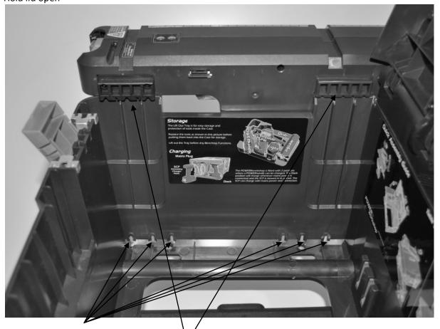
Locate and remove six (6) screws only.  $\bigvee$  Lift the charger dock up to release the hooks.
